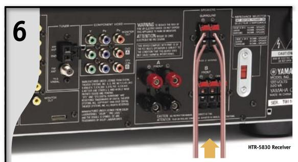
**Connect Surround Speakers** Positive (+) side of the wire with white stripe attaches to (+) terminal. Negative (-) side attaches to (-) terminal. **CAUTION** Receiver must not be plugged in while connecting speakers.
