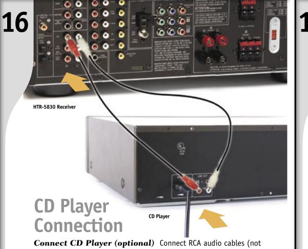
included) to "CD" terminals on receiver as shown. If your CD Player has digital output terminal, connect digital cable (not included) to HTR-5830 Receiver Digital Input terminal. See your HTR-5830 Owner's Manual for more information.
